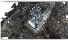
In 2017, Eye-bot Aerial Solutions, a drone service company, completed a 3D reality model of cell tower antennas in Springdale, Pennsylvania. The project team at Eye-bot initiated the Springdale Monopole project to improve model fidelity, positional accuracy, and photorealism by comprehensively modelling vertical monopole structures that feature transparent, complex cross-bracing. In the
