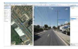
Developed by Imajing, Imajinet enables transportation infrastructure managers to host and share, within their organisation, georeferenced 3D images surveyed with the Imajbox mobile mapping system. Imajing has developed extensions to enable Imajinet integration in ArcMap with a plug-in and ArcGis Online with a widget.
