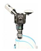
Viametris, a leader in mobile scanning technology, has announced the introduction of their new mobile scanning system for vehicles, the vMS3D. The mobile mapping system is dedicated to outdoors, roads and urban areas utilising innovative technology for localisation not dependent upon GNSS receivers and poor GNSS reception quality is no longer a problem.
