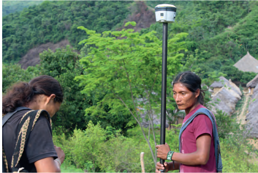
▲ Figure 6: Youngsters of the indigenous community using GNSS antennas (Trimble R2) with the village of Gunmaku visible in the background.
