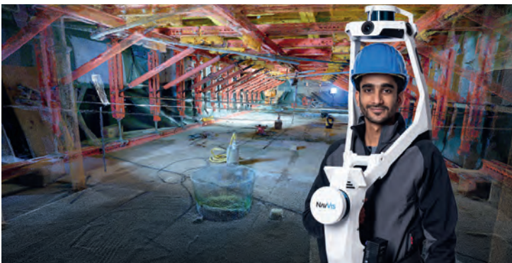
▲ NavVis VLX has both SLAM capabilities and can tie into measurement points in GNSS-denied environments.
