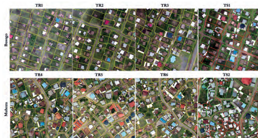
▲ Figure 4: Reference and classification maps obtained by the investigated techniques. The visible boundary references are the green lines, the invisible are the red lines, and the detected boundaries are the yellow lines. (Source: Xia X. et al., https://doi.org/10.3390/rs11141725 )
