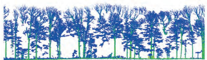
▲ Figure 4: Reconstructed Lidar data after trajectory enhancement for a terrestrial mobile Lidar.
