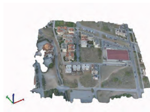
▲ Figure 2: The 3D texture mesh generated from the collected data.
