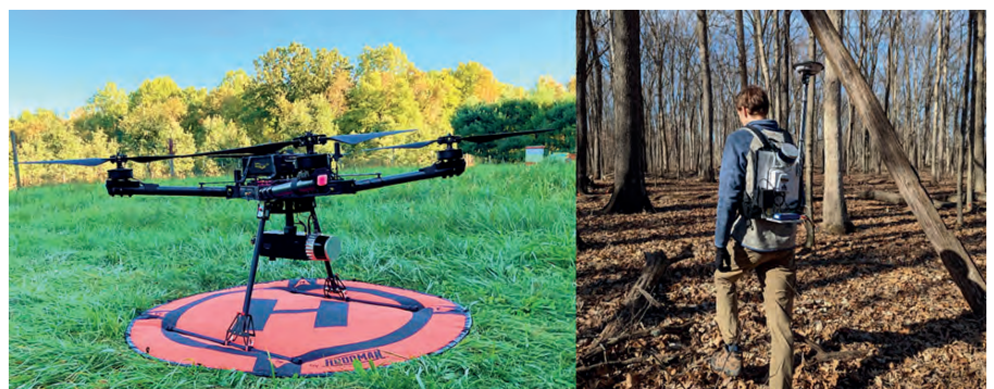
▲ Figure 1: UAV-Lidar (left) and backpack-Lidar (right) for fine-scale forest inventory.
