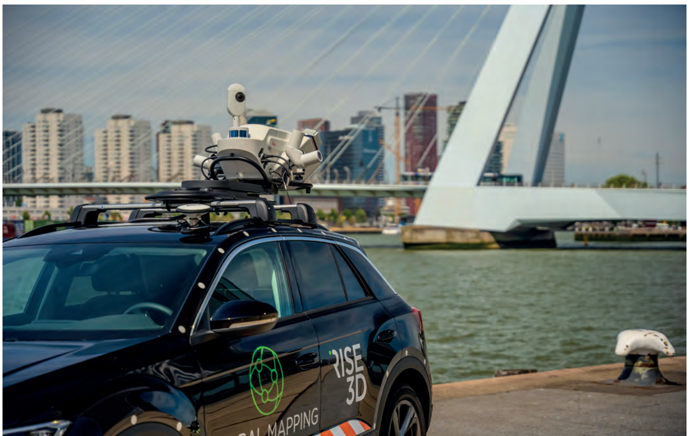
▲ A mobile mapping vehicle of Dutch digital twin specialist RISE3D on the streets of Rotterdam, the Netherlands, equipped with the Leica Pegasus TRK700 mobile mapping system.
