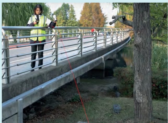
▲ Venus Laser RTK, equipped with a millimetre-level laser, eliminates the need for a range pole during stakeout and measurement, expanding the scope of work and ensuring user safety. (Image courtesy: YouTube/SinoGNSS)
