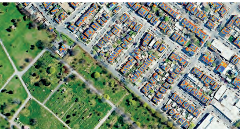
▲ Pseudo-coloured heat-loss maps of individual homes in a New York neighbourhood produced from ITRES thermal imagery. (Image courtesy: MyHeat)
