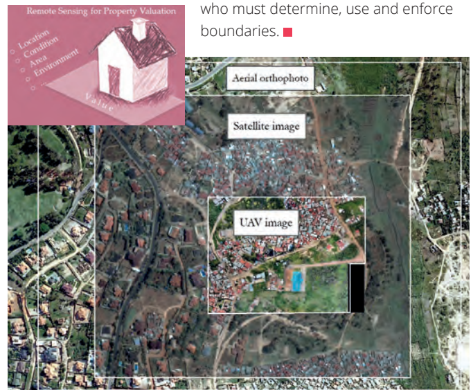
▲ Figure 7: Coverage of the remote sensing data in the Nyarutarama neighbourhood of Rwanda for property valuation based on remote sensing data. (Source: Koeva. et al., https://doi.org/10.3390/rs13183563 )
