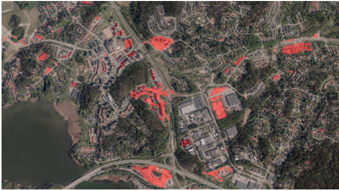
◀ Figure 4: Building and road changes recognized by the NestNet2 model (top: 2015 true orthophoto; bottom: 2020 true orthophoto).
