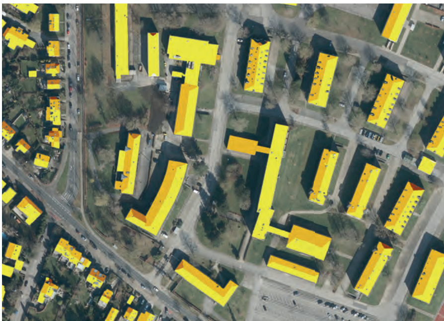
▲ Figure 3: The same buildings analysed for their solar potential, with an efficiency scale from yellow (high potential) to brown (low potential). This shows that most of the really useful areas are oriented to the south. As expected, areas that are more inclined to the north have poorer yields.
