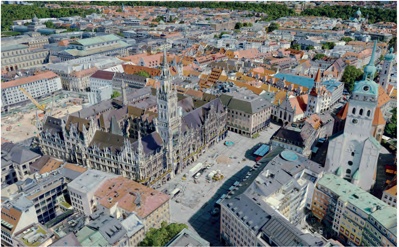
▲ 3D mesh of the city of Munich, Germany, derived by combining aerial imagery and Lidar point cloud captured with Leica CityMapper-2.
