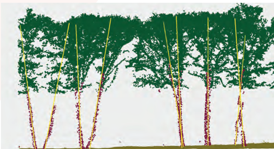
▲ The Flai solution for single tree delineation can report all relevant tree information such as tree height, canopy distribution, trunk length and radius.
