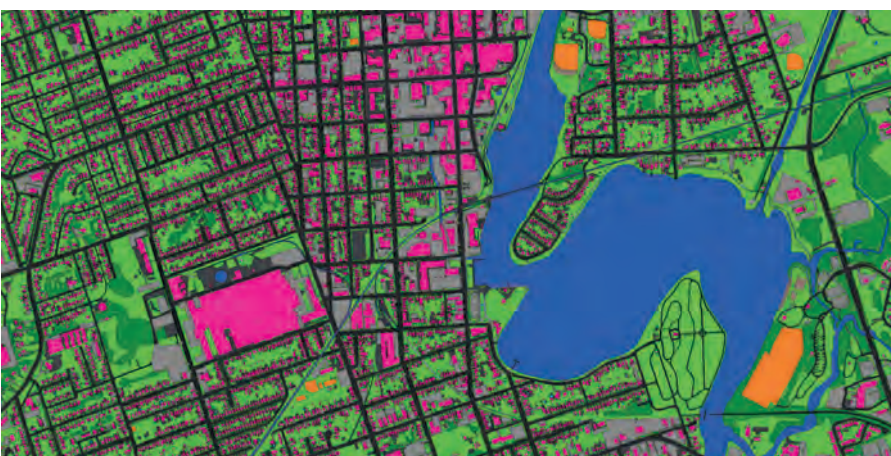
▲ Peterborough's comprehensive land cover dataset was digitized using AI for use in stormwater management.
