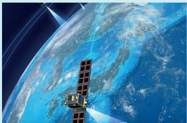
▲ StriX satellites use synthetic aperture radar (SAR) to observe and analyse the Earth's surface down to sub-metre resolutions. (Image courtesy: Synspective)
