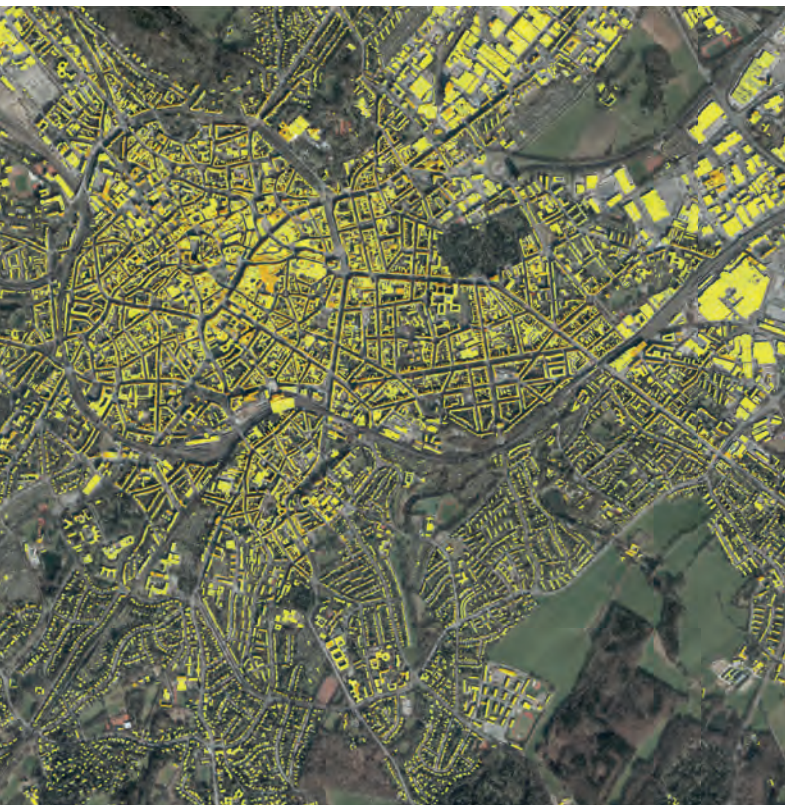
▲ Figure 4: The computed solar potential for each building in the German district of Aachen, a district with an area of around 550km 2 .
