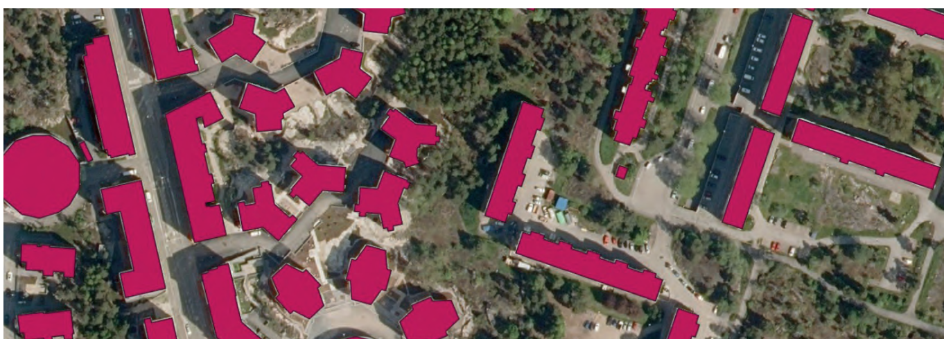
▲ Figure 3: An example of building detection from the ATMU UNet model.
