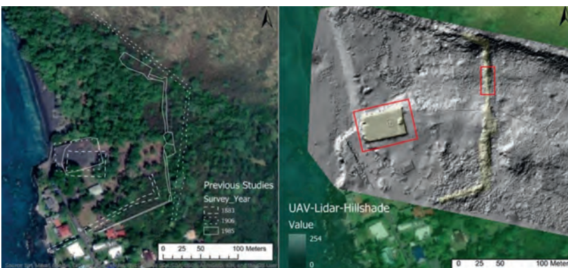
▲ Figure 4: The UAV-based Lidar survey clearly shows the current state of the largest structures at the Kealakekua Royal Centre: the temple site Hikiau Heiau and the Great Wall. Red box shows areas where terrestrial Lidar was used to measure the volume of stone used in constructing monuments. (Image courtesy: McCoy et al. 2021)
