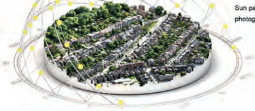
▲ Figure 7: The classified geometries extracted from the photogrammetry model.
