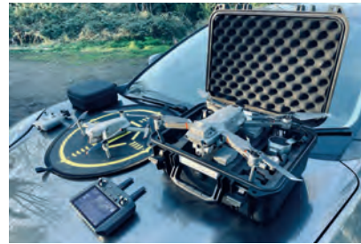
◀ Figure 1: A DJI Mavic Enterprise Advanced drone with dual lens and DJI Air 2S were used for the project.
