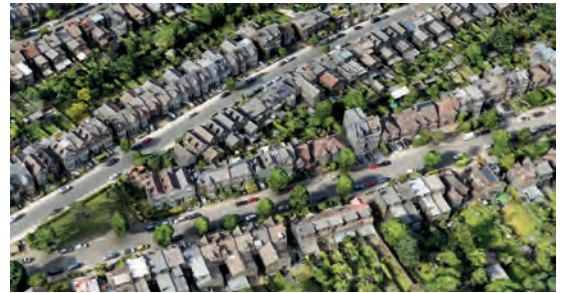
▲ Figure 8: The textured neighbourhood photogrammetry 3D model before the roofs were sorted for solar analysis.
