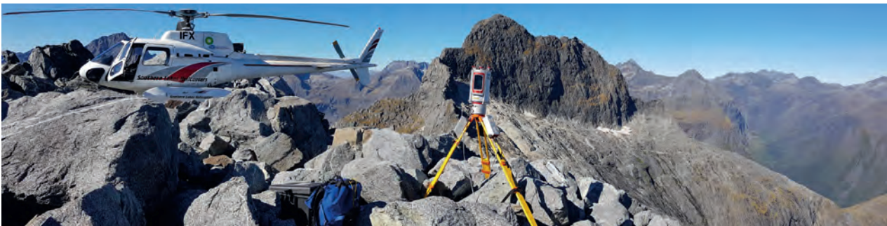
▲ Figure 3: Scanning alpine terrain (which is only accessible by helicopter) in summer. (Image courtesy: Downer Ltd, Milford Road Alliance)
