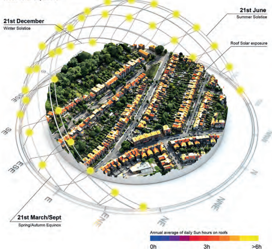
▲ Figure 4: Sun path diagram and results of the solar exposure on roofs created with Rhinoceros 3D and Grasshopper.
