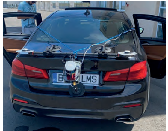
▲ Figure 6: The Lidar and INS setup ready to survey the Transylvania Ring race track.
