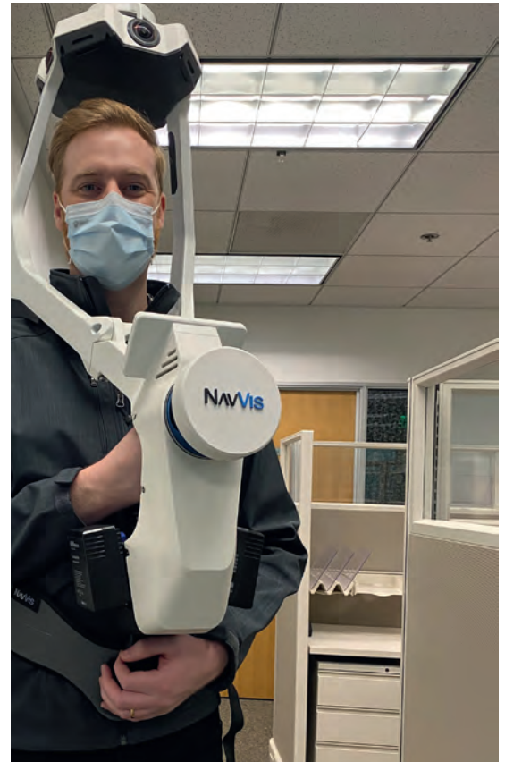
▲ With NavVis VLX, each 11-storey tower took only 10 days to scan.
