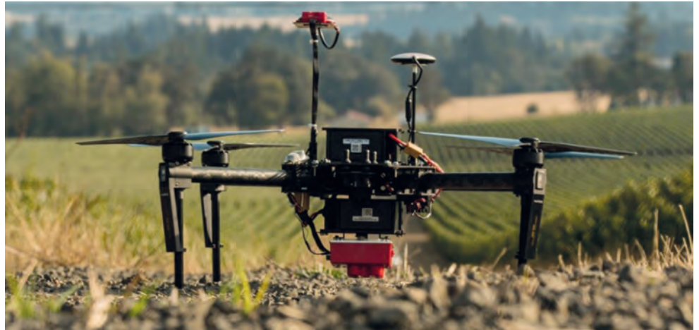
▲ Figure 4: UAV equipped with a multispectral camera. (Image courtesy: Trithi Robotics)
