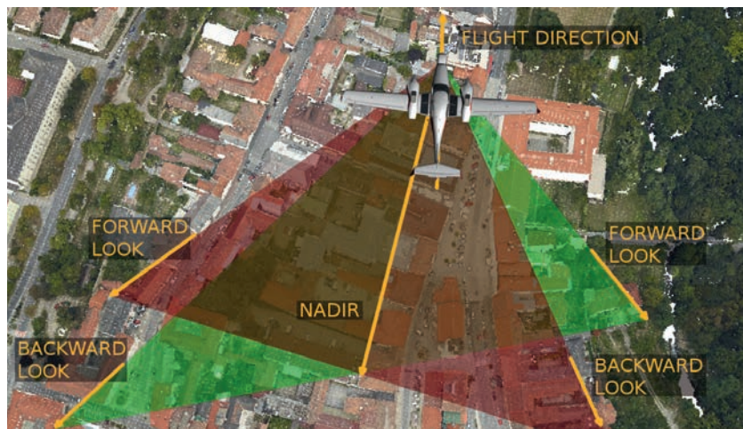
▲ Using the appropriate scanning mechanisms is crucial for specific applications. The ‘crossfire’ scan pattern of the VQ-1560 series minimizes shadowing effects in urban terrain with narrow street canyons.
