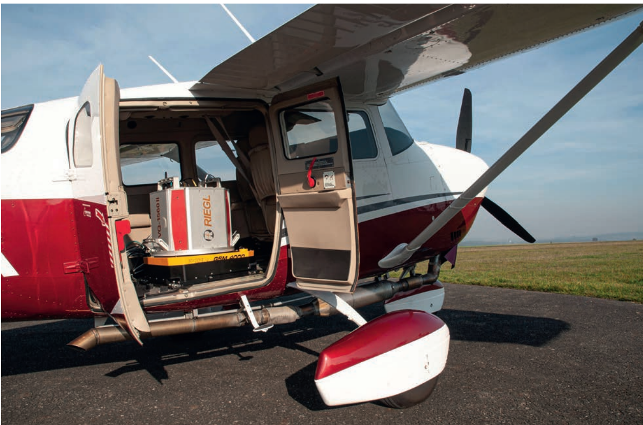
▲ A fully certified RIEGL company aircraft (a Cessna 206 with a RIEGL VQ-1560-II installed) ready for a calibration flight.
