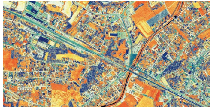
▲ A high-resolution scan with more than 50 pts/m 2 in a single pass, acquired with the VQ-1560-II from an altitude of 770m AGL at a speed of 120km/h.
