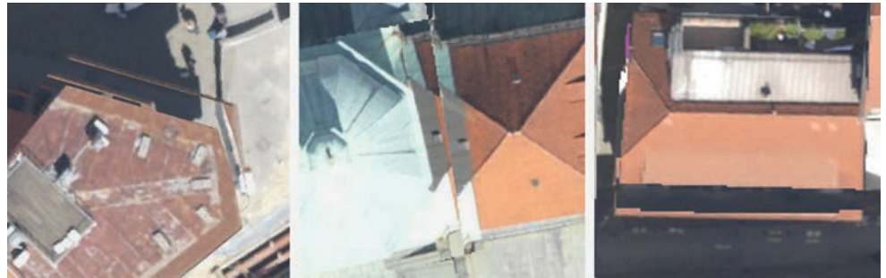
▲ Figure 2: Examples of double mapping in the true orthophoto as a consequence of inaccurately defined roof edges.
