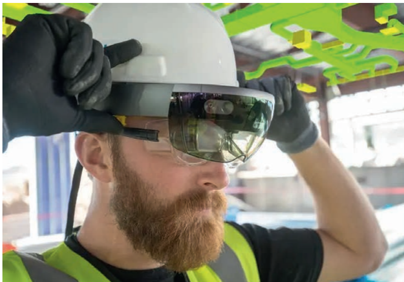
▲ Trimble's XR10 VR headset enables mixed reality to be applied in construction.
