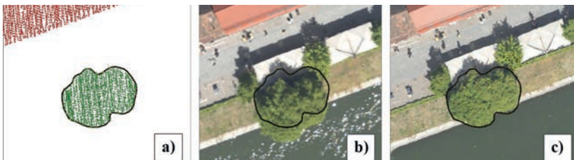
▲ Figure 5: Horizontal position of a tree: (a) vectorized from the point cloud, (b) in a true orthophoto produced from a vectorized building model, (c) in a true orthophoto produced from a digital surface model.
