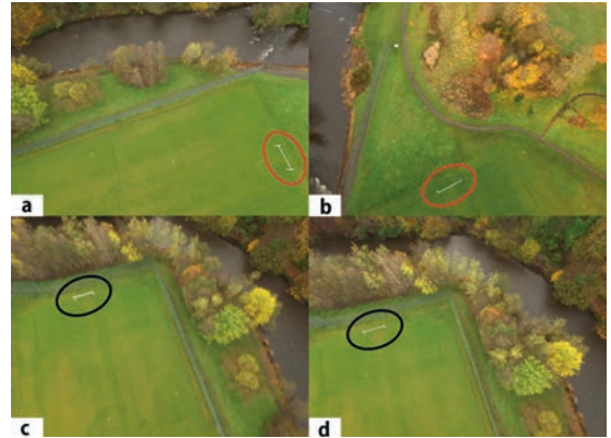
▲ A cross-section of images captured during the UAV survey showing different views of the rugby pitch and the adjoining Kelvin River. The red and black circles show regions of overlap between images a and b, and c and d respectively.
