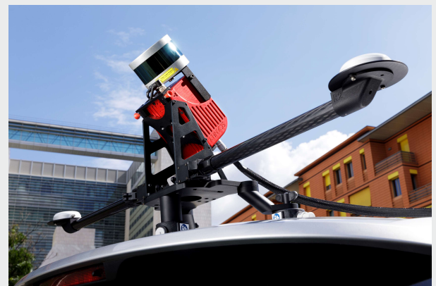
Scanfly installed on the survey vehicle
