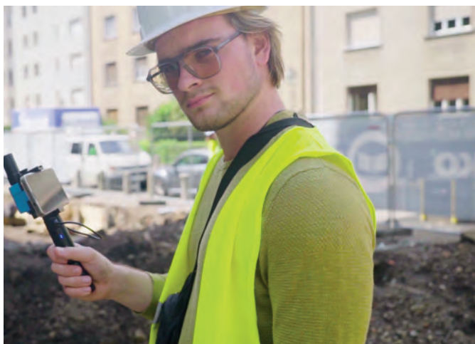
▲ Land surveyor on site with an RTK-equipped smartphone.
