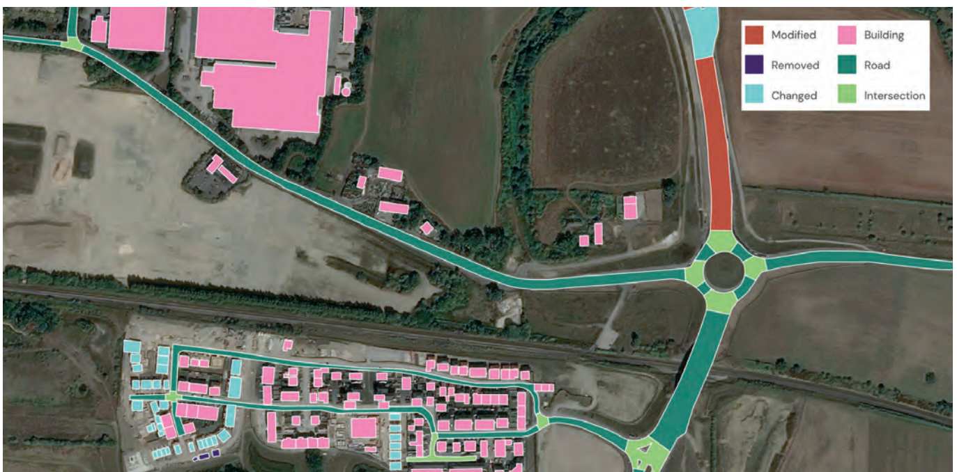
▲ Change detection map of Leeds, UK, produced in partnership with Airbus and ESA to understand the impact of land use change on railway infrastructure.
